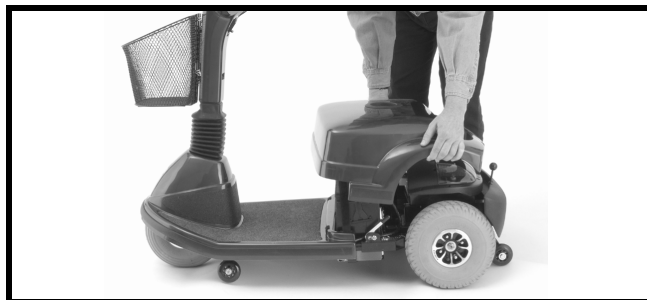
Figure 18. Rear Shroud Removal
