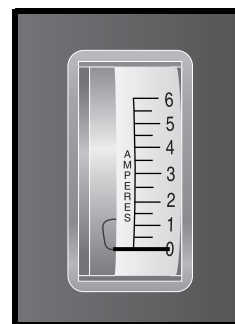
Figure 9. Ammeter Indicates Batteries Are Fully Charged
