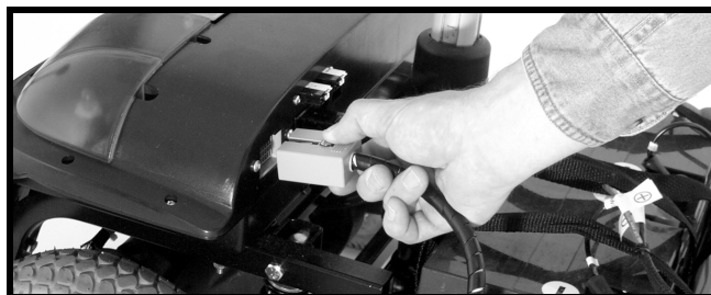
Figure 20. Disconnecting The Front-To-Rear Harness
